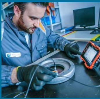
To sum it up this method allows the identification of internal defects that cause the reflection, the deviation or the absorption of an ultra sound bundle distant from transducer from a few mm to different meters.
